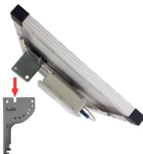
**3. Adjust the solar panel tilt angle:** set the optimal solar panel inclination according to the geographical location. The tilt angle is adjustable from 0° to 90°, with pre-defined 15° locking steps to ensure precise, reliable, and repeatable positioning.
